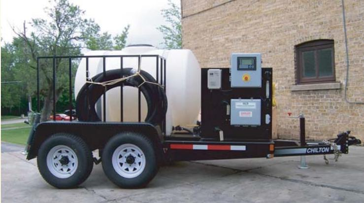
A computerized mobile fertigation system to provide proportional fertilizer injection at several irrigation sites miles apart.
